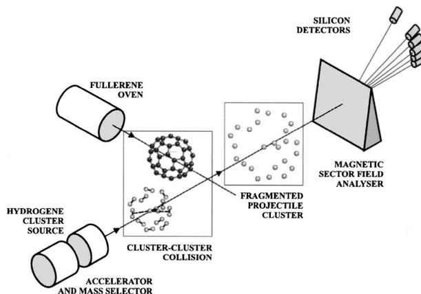
FIG. 1. A schematic view of the experimental setup.
