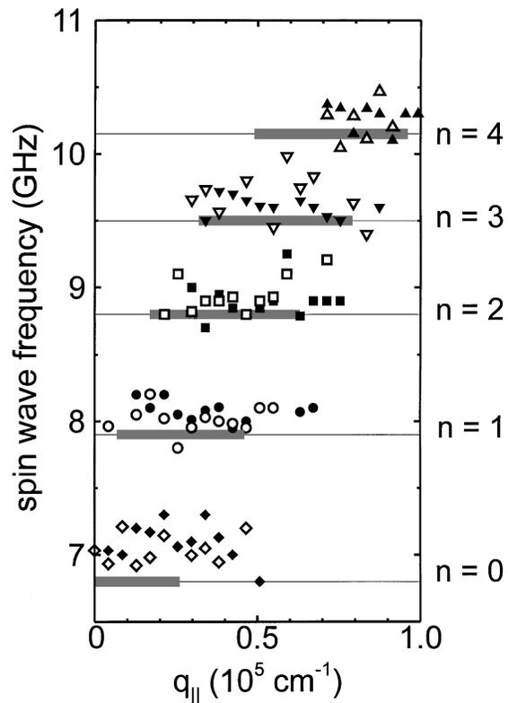
FIG. 3. Comparison of the measured mode frequencies for the wire arrays with separations of  $0.7$  μm (full symbols) and  $2.2$  μm (open symbols) with the calculated frequencies (horizontal lines), shown for the five lowest-order quantized surface spin-wave modes. The gray bars indicate the calculated wave-vector regions of observability of the discrete modes, as discussed in the text.
