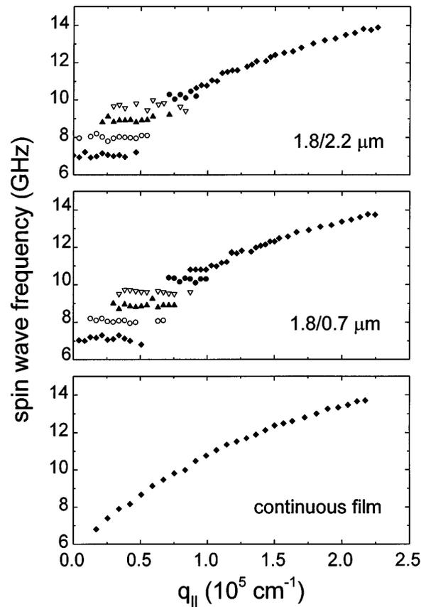
FIG. 2. Obtained spin-wave dispersion curves for an array of wires of  $1.8 \mu\text{m}$  width and a separation of the wires of  $2.2 \mu\text{m}$  (top) and  $0.7 \mu\text{m}$  (middle). The bottom panel shows a spin-wave spectrum of a continuous film for reference. The thickness of the wires and the continuous film is  $200 \text{ \AA}$ ; the external field applied along the wire axes is  $0.5 \text{ kOe}$ .
