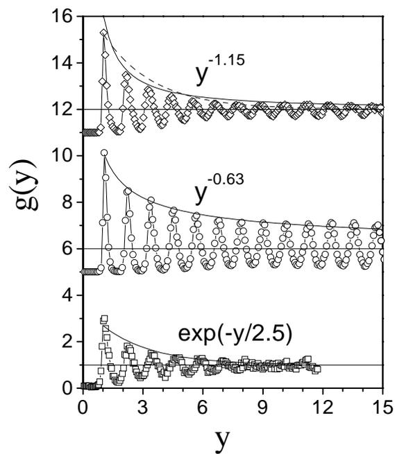
FIG. 3. Averaged pair correlation function  $g(y)$  of particles along the potential lines for  $V_0 = 0.6k_B T$  (squares),  $2.1k_B T$  (circles), and  $6.3k_B T$  (diamonds), respectively. The lines are fits as explained in the text. The data are offset in the vertical direction for clarity.
