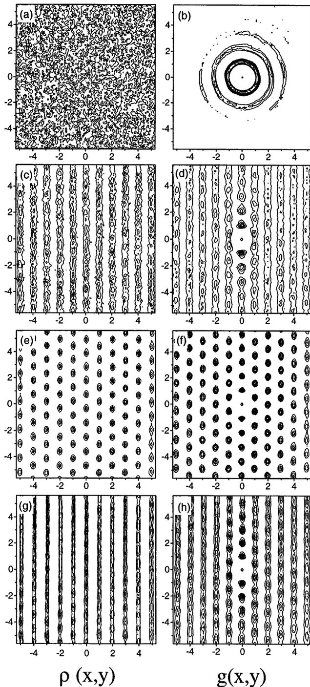
FIG. 2. Contour plots of the averaged density distribution  $\rho(x,y)$  and pair correlation function  $g(x,y)$  for zero light potential [(a),(b)] and for three nonzero potential values [{"(c),(d)  $0.6k_B T$  modulated liquid, [(e),(f)  $2.1k_B T$  crystal, and [(g),(h)  $6.3k_B T$  reentrant modulated liquid}]. The horizontal and vertical axes are  $x$  and  $y$ , respectively. All length scales are normalized by the potential period  $d$ .
