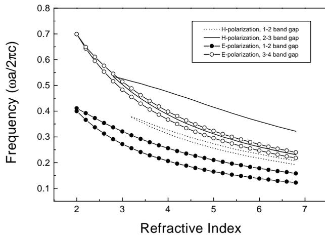
FIG. 6. Dependence of band gap positions on the refractive index for a square lattice of air cylinders in dielectric medium. The cylinders have a filling fraction of  $f = 0.7$ .
