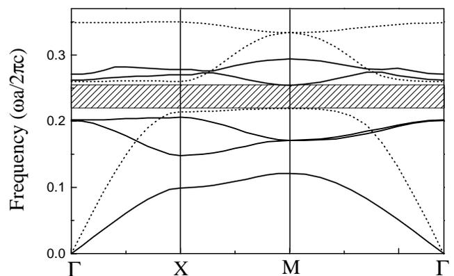
FIG. 5. Calculated photonic band structures of a square lattice of Te cylinders in air for  $E$ -polarization (solid lines) and  $H$ -polarization (dotted lines) modes. The filling fraction of Te cylinders is  $f = 0.4$ . An absolute band gap (crosshatched region) lies between  $0.219-0.254(2\pi c/a)$ .
