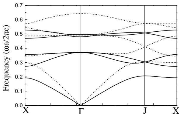
FIG. 1. Calculated photonic band structure for a triangular lattice of isotropic dielectric cylinders in air for  $E$ -polarization (solid lines) and  $H$ -polarization (dotted lines) modes. The cylinders have a refractive index of  $n = 3.6$  and a filling fraction of  $f = 0.4$ .
