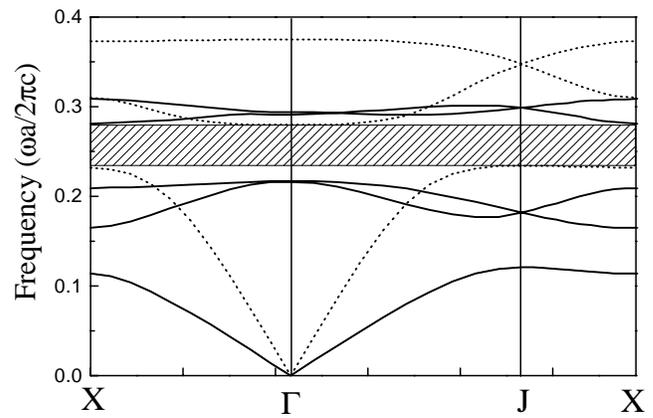
FIG. 4. Calculated photonic band structures of a triangular lattice of Te cylinders in air for  $E$ -polarization (solid lines) and  $H$ -polarization (dotted lines) modes. The filling fraction of Te cylinders is  $f = 0.4$ . An absolute band gap (crosshatched region) is present between  $0.234-0.280(2\pi c/a)$ .
