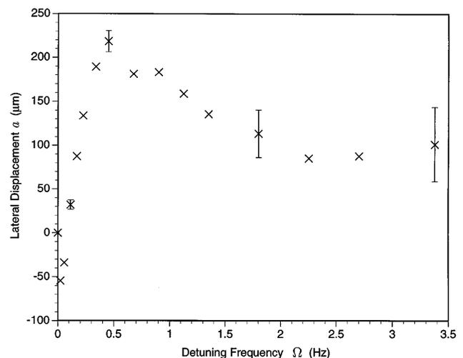
FIG. 3. Measured lateral displacement  $a$  of the conjugate-beam centroid as a function of the probe-beam detuning frequency  $\Omega$ .
