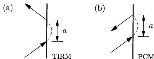
FIG. 1. Simplified illustrations of the Goos-Hänchen effect with lateral displacement  $a$  in (a) a total-internal-reflection mirror (TIRM) and (b) a phase-conjugate mirror (PCM). Beam centroids and propagation directions are represented by the arrows and flow within the mirrors is represented by the dotted curves.
