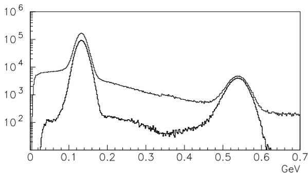
FIG. 1. Upper curve: invariant mass for  $2\gamma$  events calculated from the BGO response. Two peaks are clearly visible at the  $\pi^0$  and  $\eta$  masses before kinematical cuts. Lower curve: invariant mass for  $2\gamma$  after kinematical cuts. The resolution on the  $\eta$  mass is 50 MeV FWHM.
