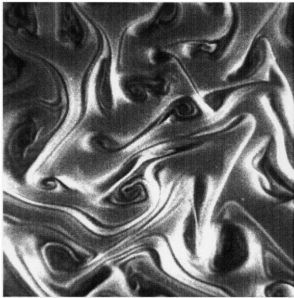
FIG. 1. Thickness field (dark is thinner, light is thicker; peak variation of \pm 35\% mean thickness) of a 2.5 \text{ cm} \times 2.5 \text{ cm} portion of the film just behind the grid.
