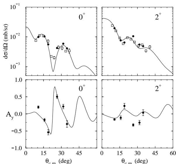
FIG. 1. Angular distributions of  $d\sigma/d\Omega$  and  $A_y$  for the  ${}^{58}\text{Ni}({}^6\text{Li}, d){}^{62}\text{Zn}$  reaction at  $E({}^6\text{Li}) = 34$  MeV leading to the  $0^+$  g.s. and the  $2^+$  first excited state. The open squares ( $\square$ ) are from Ref. [19]. The solid curves are the results of finite-range DWBA calculations described in the text.
