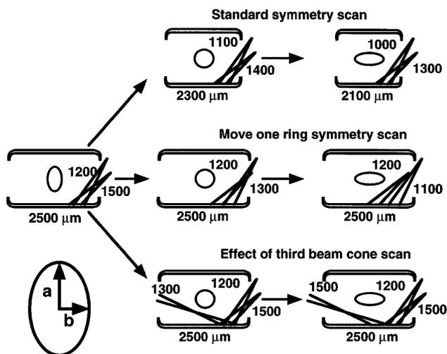
FIG. 3. Schematic showing the three types of symmetry scan performed in this experiment and the expected effect on the shape of the imploded core.
