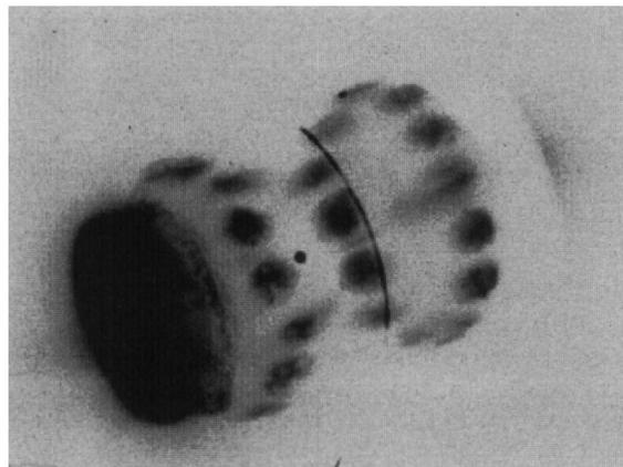
FIG. 2. X-ray pinhole camera image of a thin-wall hohlraum implosion target. The core of the imploded capsule at the center of the hohlraum is clearly seen, as are the joint in the hohlraum midplane made when mounting the capsule, the beam spots, and one laser entrance hole on the left.
