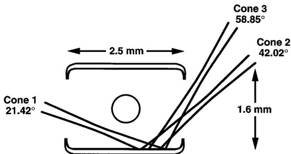
FIG. 1. Target design and typical beam pointing for the indirect-drive symmetry experiments on Omega.
