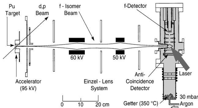
FIG. 1. Experimental setup. The primary beam hits the  $^{242}\text{Pu}$  target under an angle of  $45^\circ$ . The fission isomers recoiling out of the target are accelerated and focused with a Einzel-lens system onto the optical buffer gas cell. The gas was purified using getter techniques to a 0.1 ppm level to avoid molecule formation of americium recoils with gas impurities.
