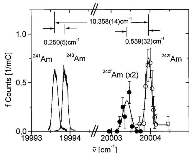
FIG. 3. Resonance ionization signals at the 500.02 nm transition of the fission isomers  $^{240,242}\text{Am}^f$  and the long-living reference isotopes  $^{241,243}\text{Am}$ . The count rate of  $^{240}\text{Am}^f$  is multiplied by a factor of 2. Experiment parameters for  $^{242}\text{Am}^f$ :  $T = 18 \text{ h}$ ,  $Q = 0.16 \text{ C}$ ,  $N = 62$ ; for  $^{240}\text{Am}^f$ :  $T = 25 \text{ h}$ ,  $Q = 0.28 \text{ C}$ ,  $N = 19$ .
