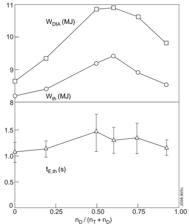
FIG. 5. (top) Diamagnetic and thermal energy contents with (bottom) the plasma energy confinement time versus DT mixture.
