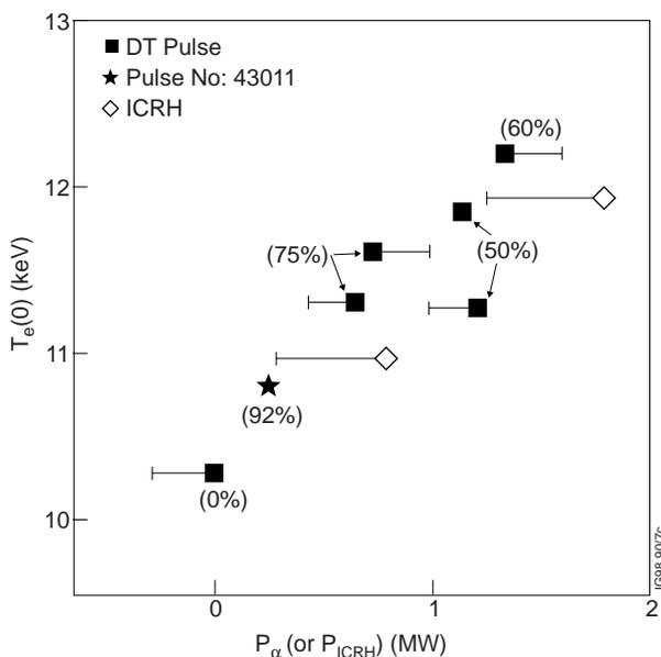
FIG. 3. Central electron temperature (ECE) versus alpha (or ICRH) power. The DT data (squares and star) and the ICRH data (open diamonds) are identified. The bars indicate the variation in NBI power compared to the 92% T pulse, 43 011. The figures in brackets are  $n_T/(n_T + n_D)$ .
