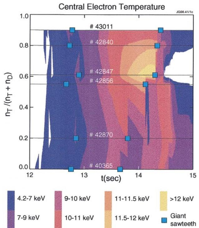
FIG. 2(color). A contour plot of central electron temperature against time (horizontal) and  $n_T/(n_T + n_D)$  (vertical) for the six pulses of the alpha heating scan. Giant sawteeth are marked with squares.
