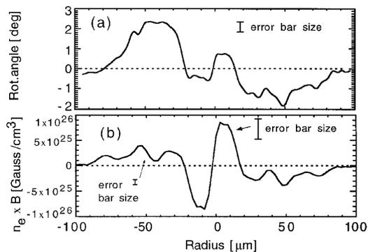
FIG. 2. (a) Faraday rotation angle obtained by microdensitometry along the arrows of Fig. 1(a). (b) Lineout of  $nB$  (density times magnetic field) extracted by Abel inversion from the trace of (a).
