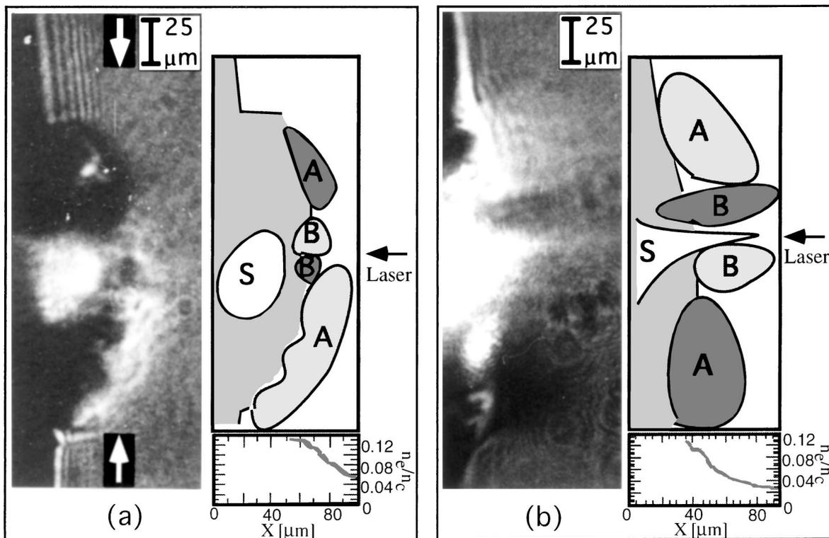
FIG. 1. Polarigrams taken (a) during the interaction of a 3 ps, 5 TW pulse with a preformed plasma (polarizers set  $-10^\circ$  off-crossed) and (b) 18 ps after the interaction of a 1.5 ps 10 TW pulse with a preformed plasma (polarizers set  $+10^\circ$  off-crossed). The on-axis density profiles of the preformed plasmas are also shown. The schematics indicate the outer (A) and inner Faraday rotation pattern (B), and the regions where self-emission is observed (S).
