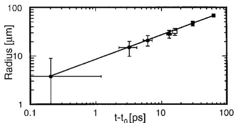
FIG. 3. Temporal evolution of the channel radius in the plasma (solid circles). The temporal axis is shifted by  $t_0 = 1.8$  ps. The solid line represents the best fit to the data using the function  $R = K(t - t_0)^{0.5}$ . The spatial extent of the inner magnetic field in the polarigram of Fig. 1(b) is also shown (empty square).
