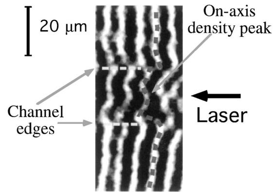
FIG. 5. Detail of an interferogram taken 5 ps after the interaction, in the conditions of Fig. 1(b). The positive fringe shift at the center of the channel is consistent with a density peak on axis.
