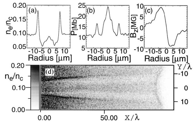
FIG. 4. 3D PIC code prediction. (a)–(c): Radial lineout at a background density of  $0.1n_c$  after 2 ps for (a) density, (b) pressure, and (c) magnetic field. (d) Longitudinal 2D section of the electron density.
