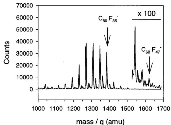
FIG. 1. Magnet scan showing relative intensity of ions extracted from the ion source.
