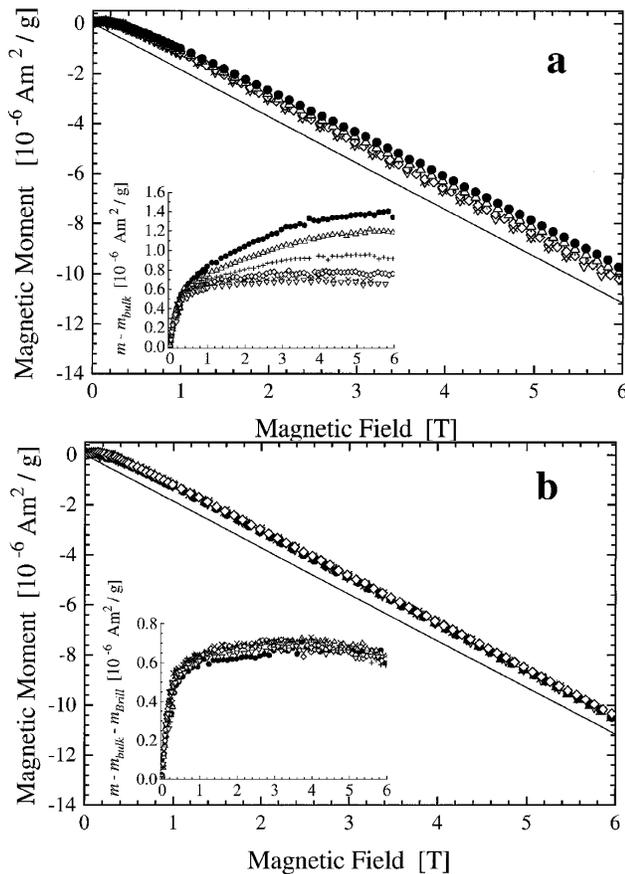
FIG. 1. (a) Field dependence of the magnetic moment of a 40 nm Ag sinter at: ( $\bullet$ ) 5 K, ( $\triangle$ ) 10 K, ( $+$ ) 20 K, ( $\diamond$ ) 50 K, ( $\times$ ) 100 K, ( $\nabla$ ) 300 K. Inset: Data after subtraction of the bulk Ag moment. (b) Data of (a) corrected for the contribution of localized paramagnetic impurities. Inset: Data after subtraction of the bulk Ag moment. The solid lines represent the data measured for bulk Ag.
