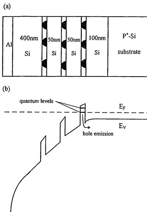
FIG. 1. Schematic diagram of the sample structure (a), and its valence band diagram under zero bias voltage (b).
