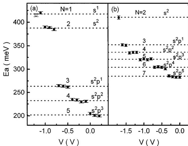
FIG. 3. The activation energies under different bias voltages of samples with typical Ge dot sizes of (a) 13 nm and (b) 25 nm.
