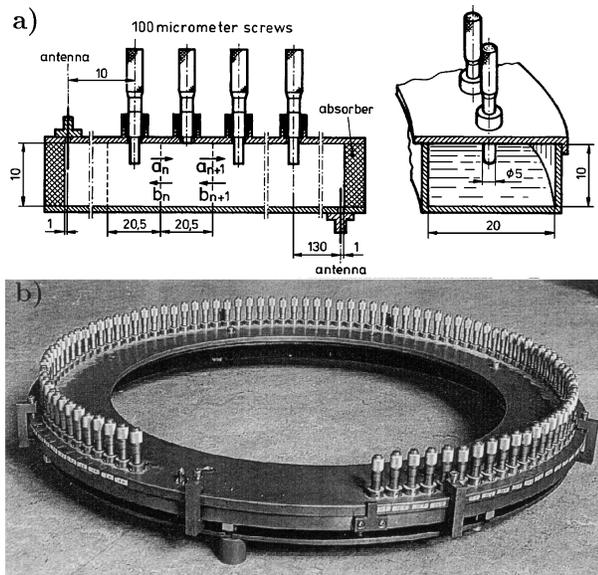
FIG. 1. (a) Schematic view of the waveguide ( $a = 20$  mm,  $b = 10$  mm). The microwaves are coupled in through the left antenna, and the transmission through the waveguide with 100 scatterers (micrometer screws) is measured with the right antenna. At each end the waveguide is closed by microwave absorbers. (b) Photograph of the apparatus.
