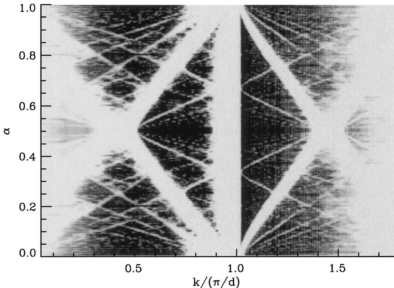
FIG. 4. Transmission spectra for a periodic arrangement of scatterers with  $\alpha$  ranging from 0 to 1 in steps of 0.005. The upper part was obtained by reflection. All 100 scatterers were used. The first two Bloch bands are seen, showing two copies of the Hofstadter butterfly. The spectra were converted to a grey scale, where black and white corresponds to high and low transmission, respectively.
