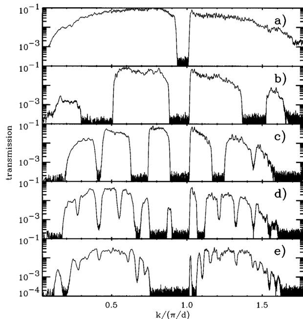
FIG. 3. Transmission spectra for different periodic arrangements with  $\alpha = 1/q$ , where  $q = 1$  (a),  $2$  (b),  $4$  (c),  $8$  (d), and  $16$  (e). In (a) the two main Bloch bands can be seen, each of which splits into  $q = 2$  subbands in (b). For larger values of  $q$  further band splitting is observed, but due to the strong absorption in the system not all  $q$  subbands can be seen.
