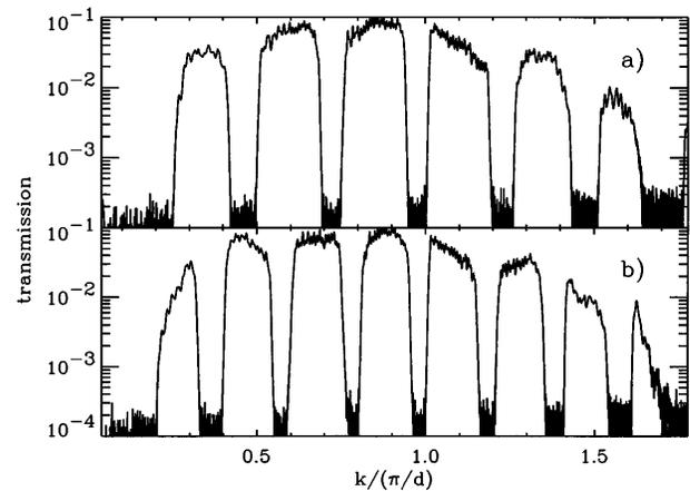
FIG. 2. Transmission probability for a periodic scatterer arrangement showing the forbidden and allowed Bloch bands. In (a) every third and in (b) every fourth scatterer was introduced 3 mm. The shown wave number range corresponds to the frequency range from 7.5 to 15 GHz.
