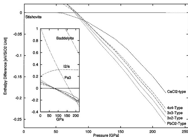
FIG. 2. Enthalpies of silica structures relative to the enthalpy of stishovite as a function of pressure. The inset considers a wider enthalpy range.
