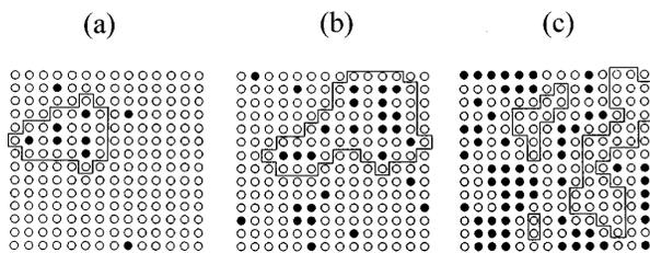
FIG. 2. Examples of fiber damage at the maximum stress in a 196 element array: (a)  $m = 10$ ; (b)  $m = 5$ ; (c)  $m = 3$ ; (broken fibers = ●, unbroken fibers = ○). Estimated critical damage clusters are constructed by using (i) breaks within next nearest neighbor distance of another break in the cluster, (ii) unbroken near neighbor elements of these breaks, and (iii) unbroken elements having two breaks at the next neighbor distance.
