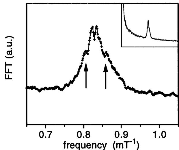
FIG. 5. The peak of the average Fourier spectrum: the splitting is evident, as well as some structure on the sides (pointed by the arrows). The inset shows the same curve on a larger frequency range: note the presence of  $1/f$  noise resulting from the switching events.
