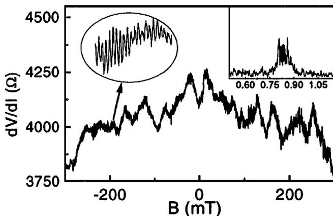
FIG. 2. Single magnetoresistance trace measured in the AB ring discussed in the text. The insets show an enlargement of the conductance oscillations and the peak in their Fourier spectrum ( $x$  axis units are in  $\text{mT}^{-1}$ ).
