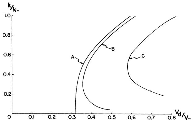
FIG. 1. Boundary between growing waves and damped waves for electron-hole plasma in InSb, with  $(m_{+}/m_{-}) = 14$ ,  $(T_{-}/T_{+}) = 10$ . Curve A represents the boundary when hole-impurity scattering is neglected, Curve B the case for  $\omega_{+}\tau_{+} = 100$ , Curve C the case for  $\omega_{+}\tau_{+} = 10$ ;  $\omega_{+} = (4\pi n_{+} e^2 / m_{+} \epsilon_0)^{1/2}$  and  $\tau_{+}$  is the lifetime of a hole against impurity scattering.
