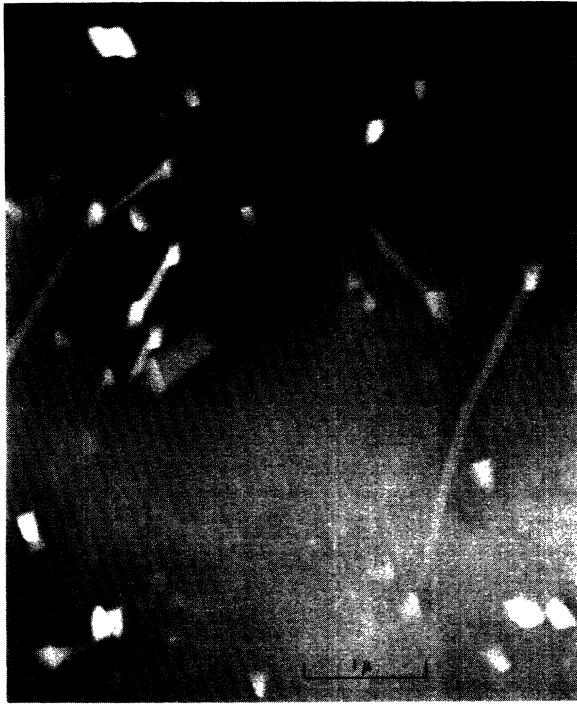
FIG. 2. Recoil nuclei tracks in etched synthetic mica. The mica was immediately adjacent to a copper foil which was bombarded with \sim 3 \times 10^{14} p/cm^2 . Etch pits as well as continuous tracks are formed. The prominent bent track probably represents a scattering event.
