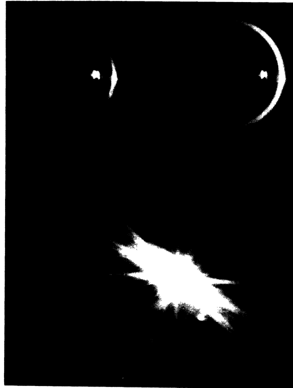
FIG. 2. Photographs of angular distribution of harmonic \nu_2 emission. Above, \psi_1 = 50.9^\circ ; below, \psi_1 = 49.6^\circ \cong \psi_0 ; the angular diameter of the ring in the above photographs is 3.9^\circ . Each photograph was obtained with one flash ( \sim 1 joule) of the ruby maser.
