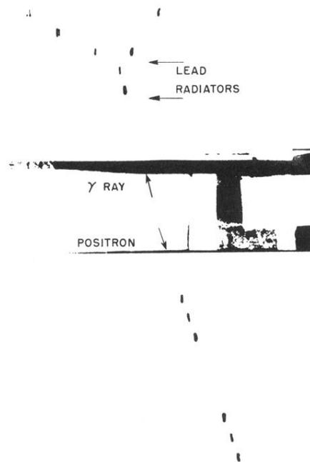
FIG. 2. Spark-chamber photograph of a radiative decay:  $\mu \rightarrow e + \gamma + \nu + \bar{\nu}$ . In the  $\gamma$  chamber, the first gap does not fire, but the  $\gamma$  ray is converted in the first lead radiator, and the resultant pair scatters to a wider opening angle in the second lead plate.
