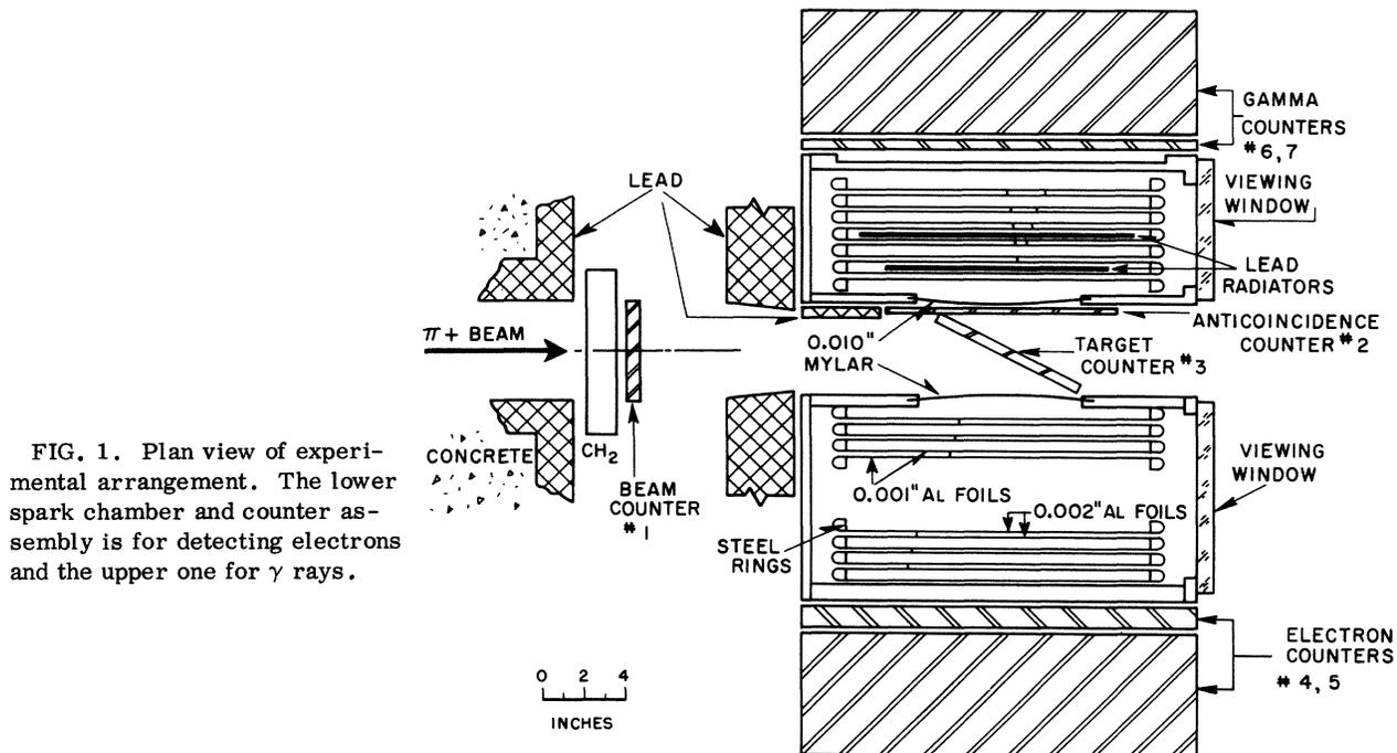
FIG. 1. Plan view of experimental arrangement. The lower spark chamber and counter assembly is for detecting electrons and the upper one for  $\gamma$  rays.
