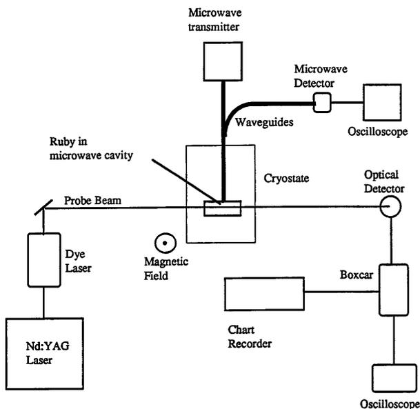
FIG. 2. Experimental setup for microwave-induced transparency in ruby.
