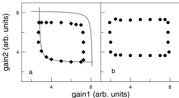
FIG. 2. Region over which control is maintained as a function of the two gains. (a) Each diode resonator was independently controlled using occasional proportional feedback control [15]. The coupling gives rise to hyperbolic boundaries. The shown hyperbolas (solid lines) are analytical results from the model assuming the eigenvalues from Fig. 1. (b) The two controllers are decoupled by *orthogonal control* resulting in a rectangular volume.
