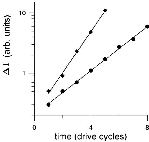
FIG. 4. Exponential departure of the peak current  $\Delta I$  from the fixed point along the two unstable eigendirections. In each graph the system was constrained to one eigendirection through orthogonal control (see text), yielding eigenvalues/slopes of 2.3 (diamonds) and 1.5 (circles).
