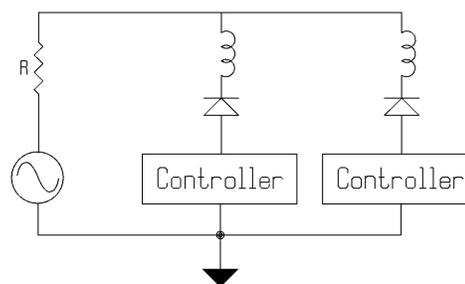
FIG. 1. The double diode resonator circuit. The coupling is provided by the resistor  $R$ . Each controller measures the deviation of the peak current through the diode from a set point and proportionally alters the respective dc bias every drive cycle.
