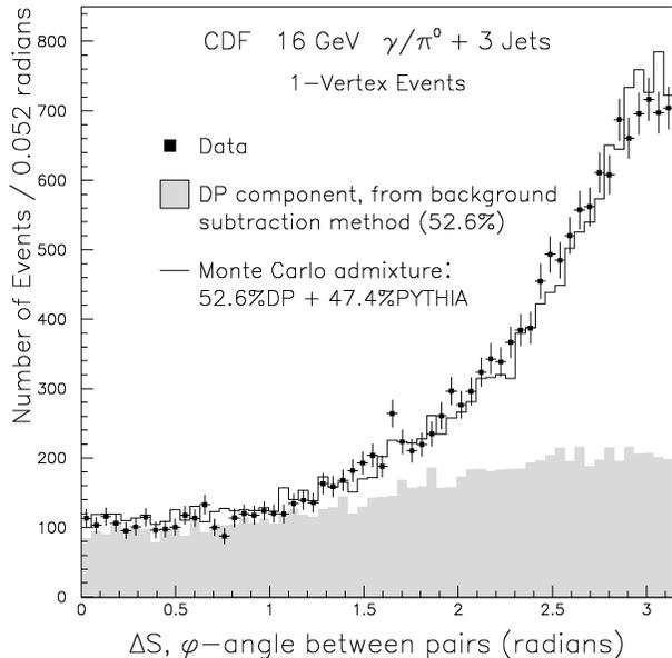
FIG. 1.  $\Delta S$  distribution for 1VTX data (points). The DP component to the data, determined by the background subtraction method to be 52.6% of the sample, is shown as the shaded region (the shape is taken from MIXDP). Also shown is the admixture 52.6% MIXDP + 47.4% PYTHIA, normalized to the data (line).
