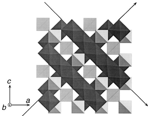
FIG. 2. Structure of  $\text{LiV}_2\text{O}_4$ . For clarity, only two layers are shown.
