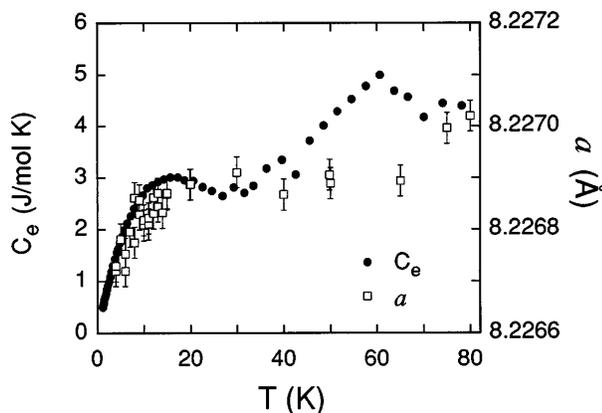
FIG. 6. Electronic specific heat  $C_e$  [1] and lattice parameter  $a$  versus temperature  $T$  below 80 K.
