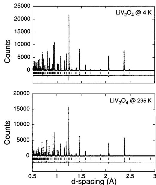
FIG. 1. Neutron diffraction data and best-fit Rietveld profile at 4 and 295 K. (+) are the observed neutron data; solid line is the calculated intensities. Tick marks show the locations of allowed Bragg peaks. The difference curve is shown at the bottom of each figure.
