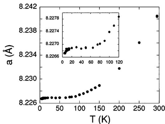
FIG. 3. Lattice parameter  $a$  as a function of temperature  $T$ .
