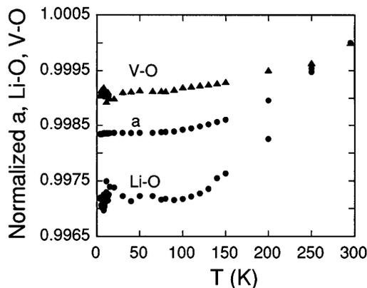
FIG. 5. Normalized lattice parameter  $a$ , and Li-O and V-O bond lengths as a function of temperature  $T$ .
