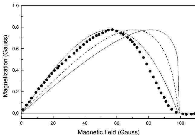
FIG. 1. Magnetization versus the external magnetic field for a superconducting disk of radius  $R = 0.315 \mu\text{m}$  and thickness  $d = 0.15 \mu\text{m}$  at  $T = 0.4$  K. Solid dots are the experimental data from Ref. [3]. We show the results of the GL theory including the 3D Maxwell equation (solid curve, and dashed curve for  $R = 0.31 \mu\text{m}$  and  $d = 0.07 \mu\text{m}$ , respectively), and the result for the LGL theory (dotted curve).
