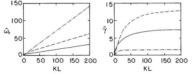
FIG. 2. Real frequency  $\hat{\omega}$  and growth rate  $\hat{\gamma}$  versus  $\hat{k}$ . Solid line (—):  $a = 0$ ,  $b = 1$ ,  $\tau^* = 40$ ,  $\hat{V} = 100$ ; dashed lines (---):  $a = 0$ ,  $b = 10$ ,  $\tau^* = 10$ ,  $\hat{V} = 10$ ; dash-dotted lines (- · -):  $a = 10$ ,  $b = 1$ ,  $\tau^* = 10$ ,  $\hat{V} = 10$ .
