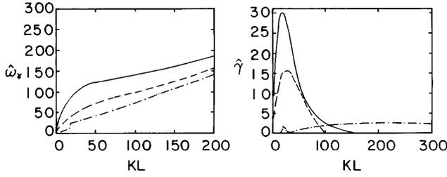
FIG. 1. Real frequency  $\hat{\omega}$  and growth rate  $\hat{\gamma}$  versus  $\hat{k}$ . Solid lines (—):  $a = 30\,000$ ,  $b = 10$ ,  $\tau^* = 1$ ,  $\hat{V} = 0$ ; dashed lines (---):  $a = 10\,000$ ,  $b = 50$ ,  $\tau^* = 1$ ,  $\hat{V} = 0$ ; dash-dotted lines (- · -):  $a = 1000$ ,  $b = 50$ ,  $\tau^* = 1$ ,  $\hat{V} = 1$ .
