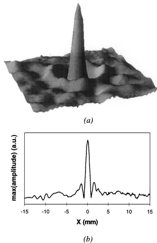
FIG. 4.  $A_0$  component of the focal spot. (a) Wave field at  $t_R = 0$  on a square of  $15 \times 15$  mm. (b) cut of the focal spot.
