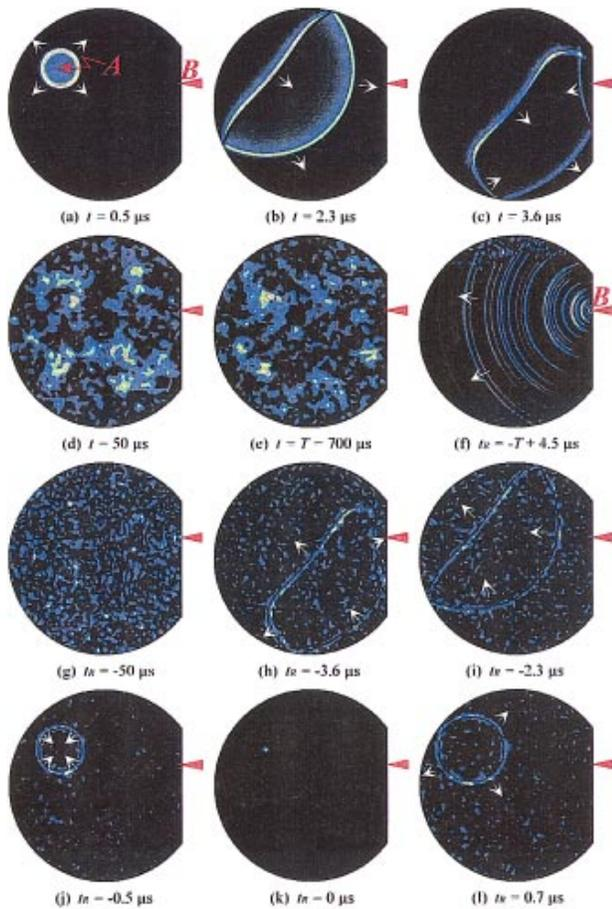
FIG. 1(color). Finite difference simulation of a one-channel time reversal. (a)–(e) Injection of a short pulse in  $A$  and recording in  $B$ . (f)–(l) Emission of the time-reversed signal in  $B$  and refocusing.
