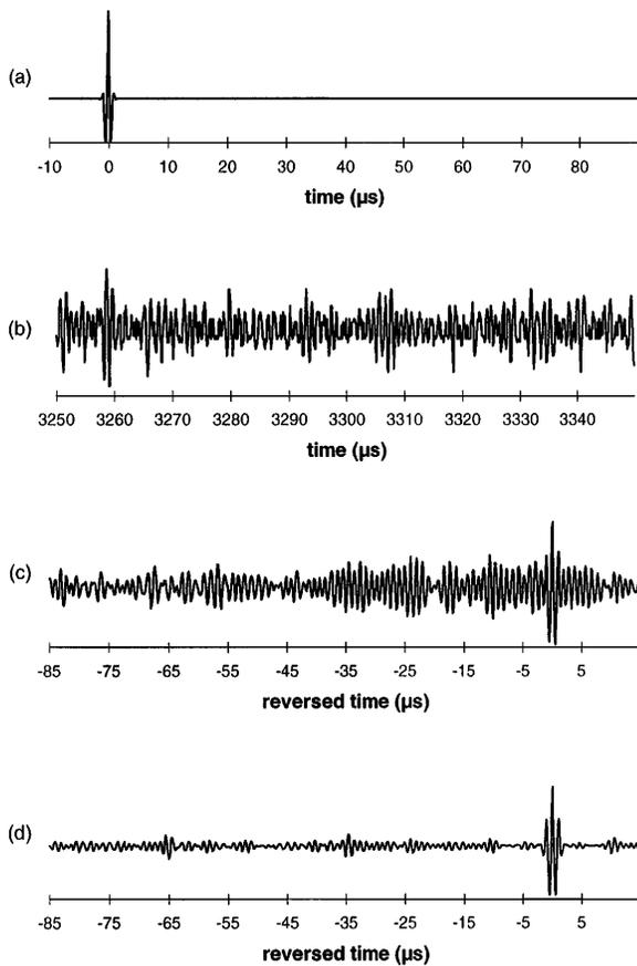
FIG. 3. Some characteristic signals. (a) Excitation pulse introduced at point *A* into the wafer. (b) Typical shape of a signal received at point *B*. (c) and (d) Typical refocusing peaks obtained at point *A*, applying a time-reversal window of  $\Delta T = 40$   $\mu\text{s}$  and  $\Delta T = 1500$   $\mu\text{s}$ , respectively.
