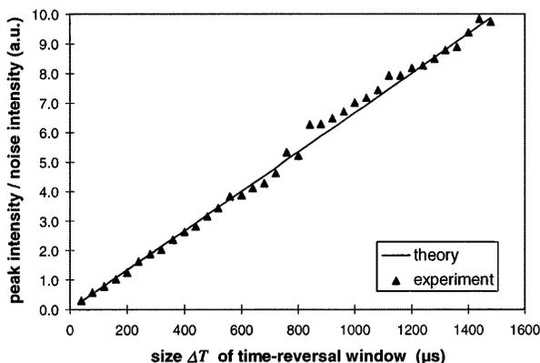
FIG. 5. Comparison of experimental and theoretical focusing quality for varying time-reversal window sizes.
