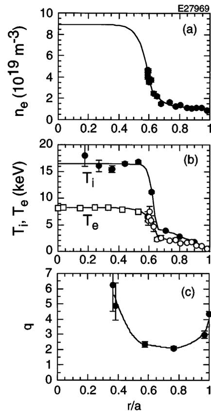
FIG. 3.  $n_e$ ,  $T_i$ ,  $T_e$ , and  $q$  profiles at  $t = 7.15$  s in which the  $T_e$  is measured by Thomson scattering (open circles) and ECE (open squares).
