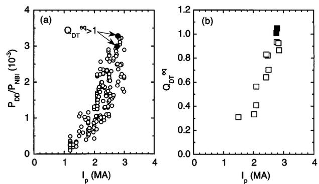
FIG. 5. (a) Ratio of the  $D$ - $D$  fusion power to  $P_{NBI}$  with  $H$  factor above 1.5 and (b)  $Q_{DT}^{eq}$  for typical high performance discharges as a function of  $I_p$  for the reversed shear discharges. Closed symbols indicate the discharges achieving  $Q_{DT}^{eq}$  in excess of unity.
