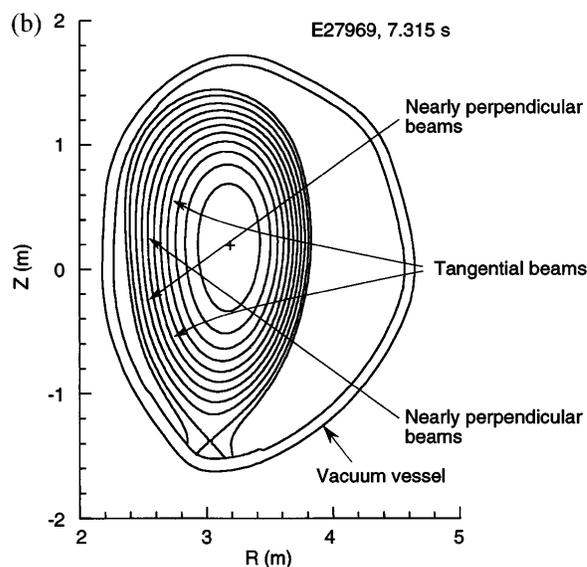
FIG. 1. (a) Discharge wave forms for E27969 with  $I_p$ ,  $P_{\text{NBI}}$ ,  $W_{\text{dia}}$ ,  $S_n$ , central and peripheral  $\bar{n}_e$ ,  $H$  factor, normalized beta ( $\beta_N = \beta_t a B_f / I_p$ ),  $T_i$ ,  $T_e$ , and  $q$  at 95% flux ( $q_{95}$ ), and magnetic pitch minimum ( $q_{\min}$ ). (b) The equilibrium configuration reconstructed using the motional Stark effect (MSE) data along with the injection paths of neutral beams.
