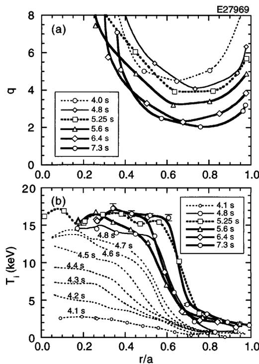
FIG. 2. Evolution of the safety factor ( $q$ ) and  $T_i$  profiles for E27969, which are measured from the MSE spectroscopy and the charge exchange recombination spectroscopy, respectively.
