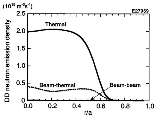
FIG. 4. Calculated profiles of  $D$ - $D$  neutron emission density at  $t = 7.315$  s for E27969 showing the thermal, beam-thermal, and beam-beam components.
