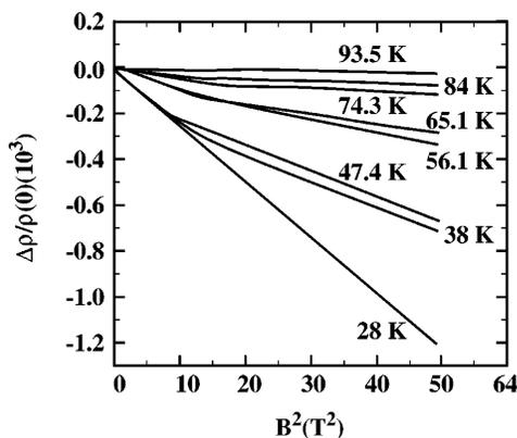
FIG. 4. Magnetic field dependence of the magnetoresistance for an  $\text{YH}_{2.99}$  film [see Fig. 2(b)] at the indicated temperatures. Above 100 K the magnetoresistance vanishes within experimental errors. The magnetic field is applied perpendicular to the current and the plane of the film. Essentially the same results are obtained for a field perpendicular to the current but parallel to the plane of the film.
