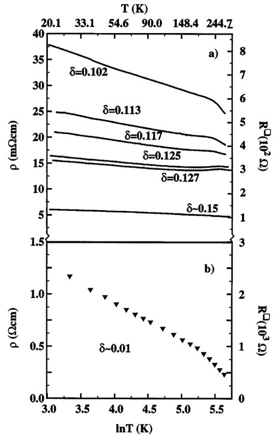
FIG. 2. Logarithmic temperature dependence of the electrical resistivity  $\rho$  and the resistance per square  $R^\square$  which is observed in the  $\text{YH}_{3-\delta}$  films in regime III (see Fig. 1). In (a) the increase of the logarithmic slope with decreasing hydrogen deficiency  $\delta$  is illustrated. As shown in (b), the logarithmic temperature dependence clearly persists for a high resistivity film with an hydrogen deficiency as small as 0.01.
