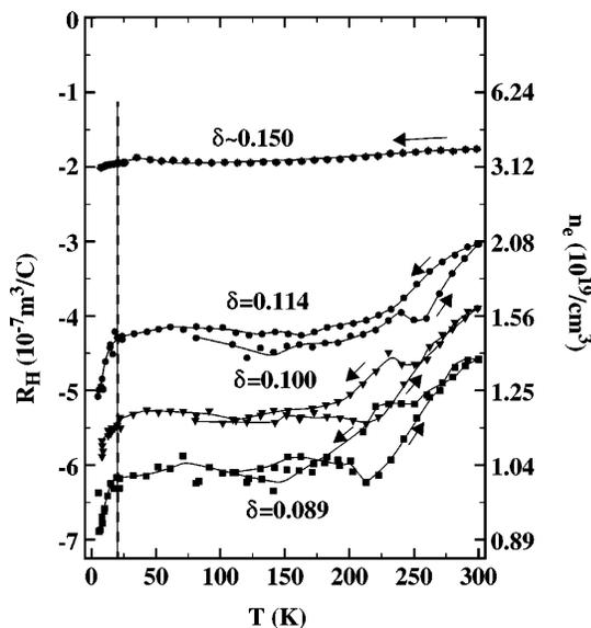
FIG. 3. Temperature dependence of the Hall constant  $R_H$  and of the corresponding electron density  $n_e = -1/(R_H e)$  in a  $\text{YH}_{3-\delta}$  films for four different values of the hydrogen deficiency  $\delta$ . The hysteresis near 225 K is due to the order-disorder transition (see regime II in Fig. 1). Below 20 K (corresponding to regime IV in Fig. 1) the carrier density starts to decrease.
