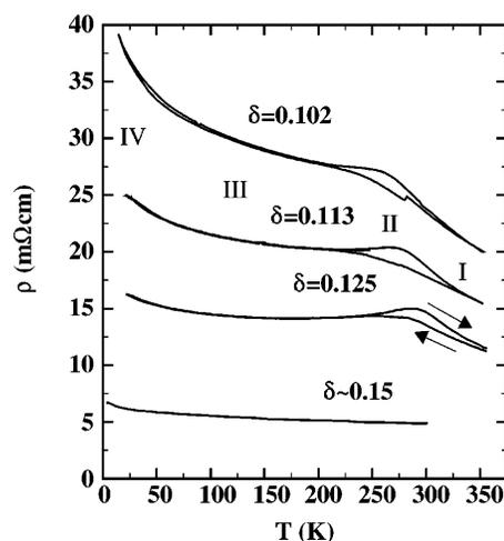
FIG. 1. Temperature dependence of the resistivity  $\rho$  in a 500 nm thick  $\text{YH}_{3-\delta}$  film for four different values of the hydrogen deficiency  $\delta$ . Four temperature regimes labeled I to IV can be distinguished (see text). The hysteresis in regime II is due to the order-disorder transition.
