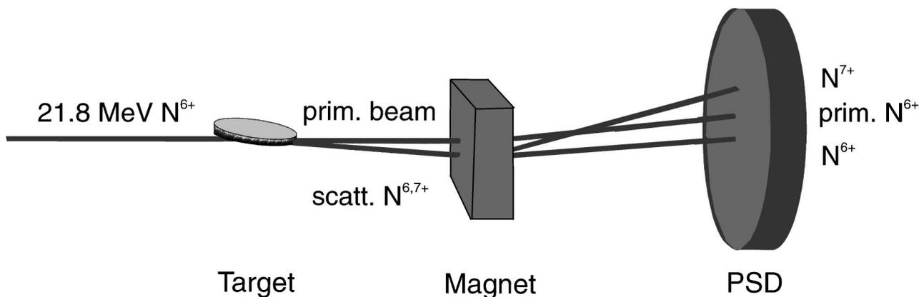
FIG. 1. Sketch of the experimental setup with target, magnet, and position sensitive detector (PSD). The trajectories of the primary beam and the scattered  $N^{6+}$  and  $N^{7+}$  beams are shown schematically. The distance from the target to magnet is 1.7 m. The distance from target to the PSD is 2.4 m.
