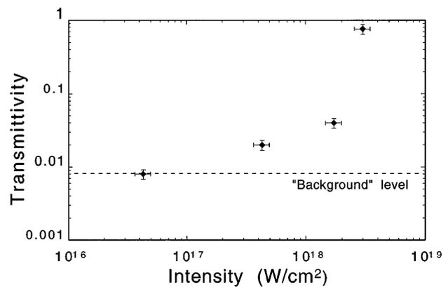
FIG. 1. Transmittivity as a function of the intensity of the 30 fs laser pulse incident on 0.1  $\mu$ m thick plastic target. The background level indicates the level at which the energy in the pedestal (ASE) is comparable with the transmitted energy.
