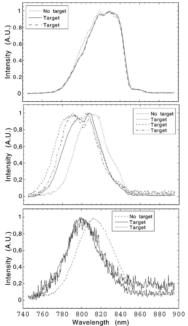
FIG. 3. Space resolved spectra of the transmitted pulse at three different intensities on target,  $3 \times 10^{18} \text{ W/cm}^2$  (upper),  $4 \times 10^{17} \text{ W/cm}^2$  (middle), and  $5 \times 10^{16} \text{ W/cm}^2$  (lower). The unperturbed laser spectrum (dotted line) obtained without the target at each laser intensity is also plotted for comparison.
