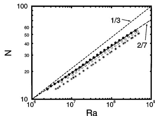
FIG. 2.  $N$  vs  $Ra$  at fixed  $Ro$ : 0.30 ( $\bullet$ ), 0.75 ( $\diamond$ ), and  $\infty$  ( $*$ ). The short dashed line and the long dashed line represent the  $1/3$  and  $2/7$  power laws, respectively.
