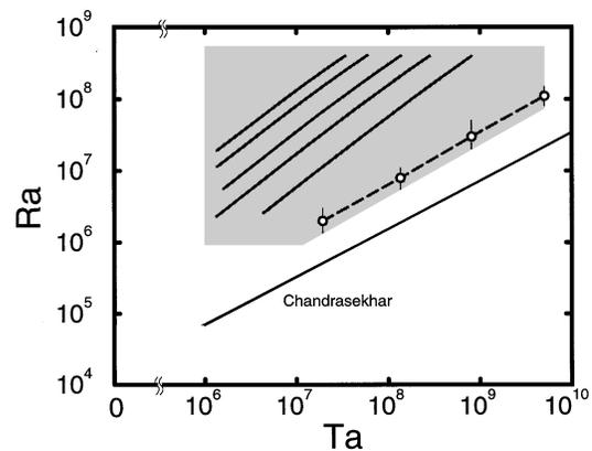
FIG. 1. Parameter space diagram  $Ra$  vs  $Ta$ . Measurements at fixed  $Ro$  were in the shaded area in which the five solid lines correspond to different values of  $Ro$  (from right to left, 0.30, 0.52, 0.75, 1.15, and 1.49). Symbols ( $\circ$ ) set the lower bound above which  $N$  exhibited approximate scaling with  $Ra$ . Theoretical prediction for onset of bulk convection under rotation is also shown [18].
