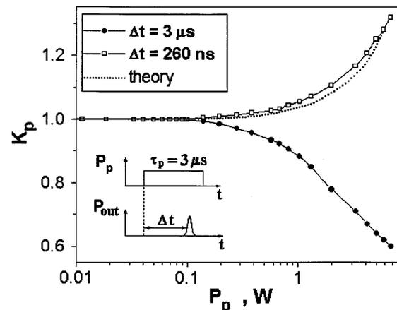
FIG. 5. Soliton amplification coefficient  $K_p$  vs pumping power  $P_p$  measured for  $P_{in} = 0.25 \text{ W}$  and two values of  $\Delta t$ :  $\Delta t_1 = 260 \text{ ns}$  and  $\Delta t_2 = 3 \mu\text{s}$ . Dotted line shows the theoretical curve calculated from Eq. (12).
