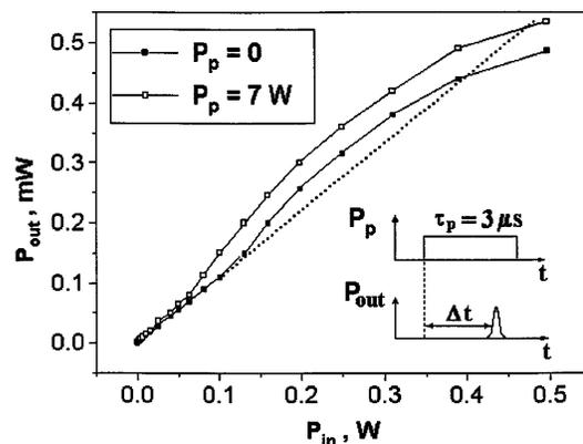
FIG. 2. Amplitude characteristics of the experimental delay line obtained with and without pumping. Dotted line shows amplitude characteristic in the linear regime. The inset shows relative positions in time of the pumping pulse and the output SW envelope soliton ( $\Delta t = 260$  ns for this experiment).
