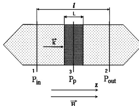
FIG. 1. Diagram of the experimental delay-line structure: 1 and 2 are the input and output transducers, 3 is the pumping transducer, and the dark region of the width  $L$  is the region of pumping localization.
