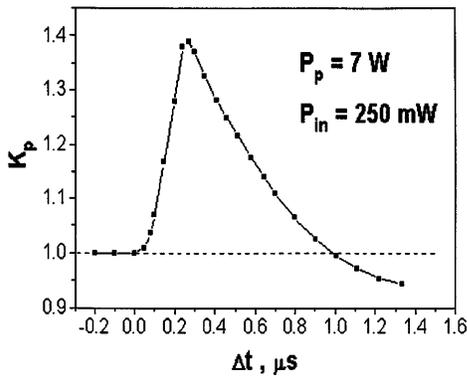
FIG. 4. Soliton amplification coefficient  $K_p$  vs time delay  $\Delta t$  between pumping pulse and the output soliton (see inset in Fig. 2) obtained for  $P_{in} = 0.25 \text{ W}$ ,  $P_p = 7 \text{ W}$ , and  $T_p = 3 \mu\text{s}$ .
