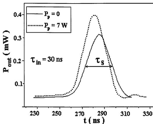
FIG. 3. Profiles of output pulses (power vs time) obtained with and without pumping for  $P_{\text{in}} = 0.25$  W, and  $\Delta t = 260$  ns.
