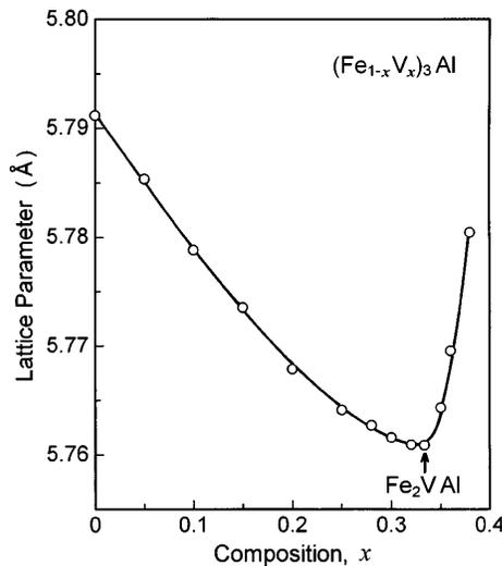
FIG. 1. Lattice parameter of the  $D0_3$  phase in  $(\text{Fe}_{1-x}\text{V}_x)_3\text{Al}$  as a function of V composition  $x$ . The arrow indicates the composition ( $x = 0.33$ ) of the Heusler-type  $\text{Fe}_2\text{VAl}$  compound.
