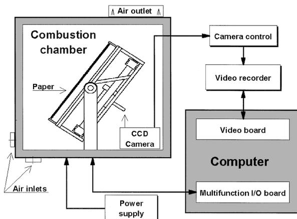
FIG. 1. A schematic diagram of the experimental setup.
