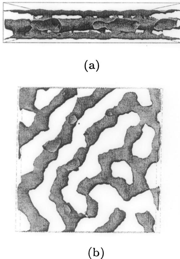
FIG. 3. The snapshot of the system configuration for  $N_z = 10$  (a) and the top view of the inside structure formed in the middle of the system (b). The system consists of two layers attached to the walls (a) and the disordered network of channels lying in the  $x$ - $y$  plane (b) ( $z$  axis is perpendicular to the walls).
