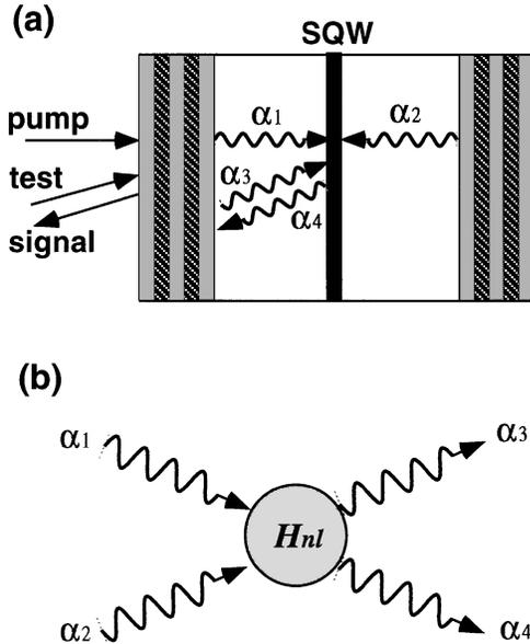
FIG. 3. (a) Schematic of the self-pumped phase conjugation experiment. (b) Relevant processes for DFWM based on the cavity-polariton picture. Two incoming polaritons provided by the pump beam are elastically scattered into two outgoing polaritons conserving energy and momentum.
