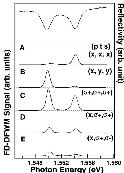
FIG. 2. Spectra of FD-DFWM at zero detuning for various polarization configurations indicated in the figure are described in the text.
