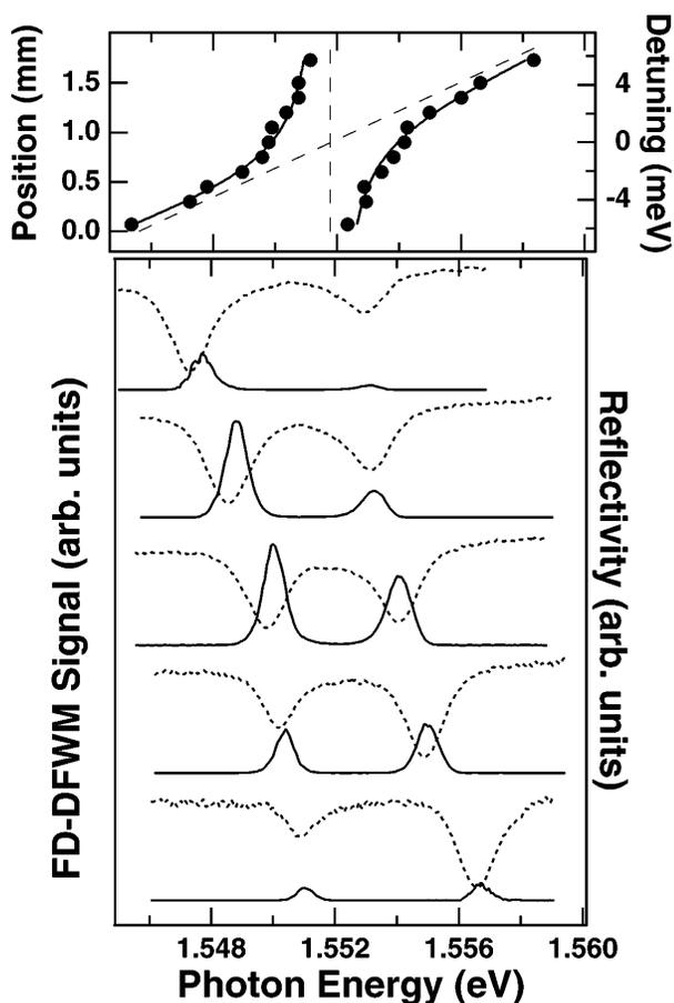
FIG. 1. Linear reflection spectra (dotted lines) and degenerate four-wave mixing spectra (solid lines) of the GaAs SQW for various detunings. DFWM measurements are performed in the co-circular polarization configuration, where all the beams are  $\sigma_+$  polarized. In the upper graph, the normal mode resonance observed in linear reflection spectra is plotted as a function of spot position. The calibrated energy scale for detuning energy is shown.
