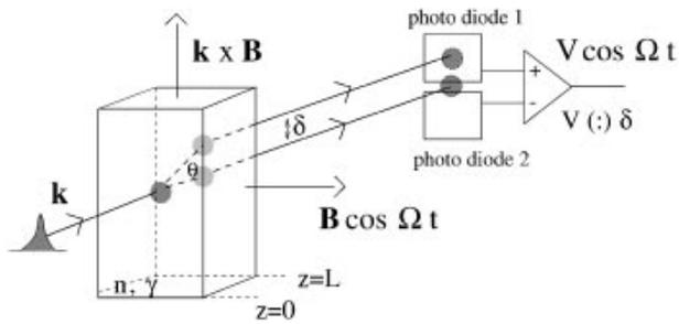
FIG. 1. Schematic setup. As shown, the displacement of the beam in the  $\mathbf{k} \times \mathbf{B}$  direction is detected. By rotating the photodiode assembly over  $90^\circ$  along  $\mathbf{k}$ , the  $\mathbf{B}$  axis displacement is detected.
