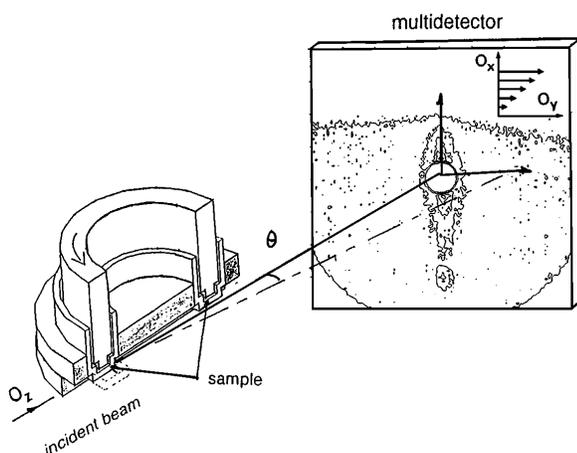
FIG. 2. Schematic of the neutron scattering cell used for the observation of the vorticity plane with a typical neutron scattering pattern ( $\lambda = 3.5 \text{ \AA}$ ,  $d = 2 \text{ m}$ ) obtained with the H/D mixture in the smectic phase ( $T = 93 \text{ }^\circ\text{C}$ ) under a shear flow of  $6 \text{ s}^{-1}$ . The upper part of the pattern corresponds to a shadow due to the upper rotating ring.
