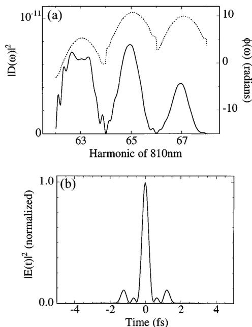
FIG. 4. (a) Part of the high harmonic spectrum for neon at 810 nm,  $4 \times 10^{14}$  W/cm<sup>2</sup> peak intensity, and 27 fs pulse width. Solid line:  $|D(\omega)|^2$ ; dotted line:  $\phi(\omega)$ . (b) Electric field envelope of the three harmonics in shown (a) after removing the average group delay.
