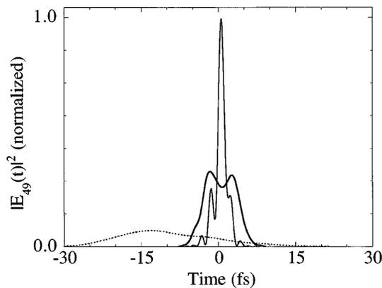
FIG. 2. Electric field envelope of the 49th harmonic at 810 nm and  $3 \times 10^{14}$  W/cm<sup>2</sup> peak intensity. The pulse duration is 108 fs (dashed), 27 fs (heavy line), or 13.5 fs (thin line).
