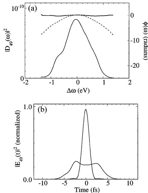
FIG. 3. (a) Envelope and phase of the 49th harmonic from Fig. 1. Initial phase (dotted line) and the phase with its quadratic component removed (upper solid line). (b) Electric field envelope of the 49th harmonic before and after compression.
