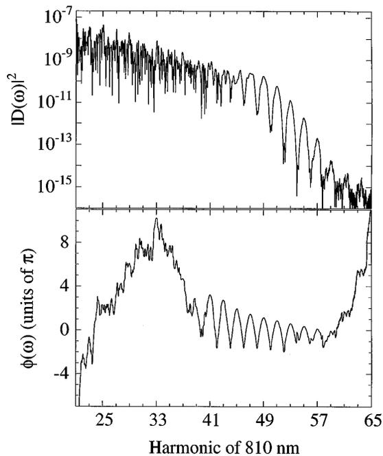
FIG. 1. Argon at 810 nm,  $3 \times 10^{14}$  W/cm<sup>2</sup> peak intensity and 27 fs FWHM pulse width. Upper panel:  $|\mathcal{D}(\omega)|^2$ ; lower panel:  $\phi(\omega)$ .
