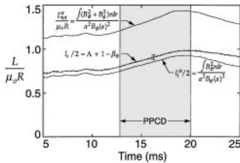
FIG. 4. Normalized inductances for ensemble data of Fig. 3. Superscript “ $\alpha$ ” indicates equilibrium model predictions [Eq. (2)]. For better illustration of the time evolution, this comparison is shown for fixed  $\beta_\theta = 10\%$ . [The temporal resolution of  $\beta(t)$  is coarse.]
