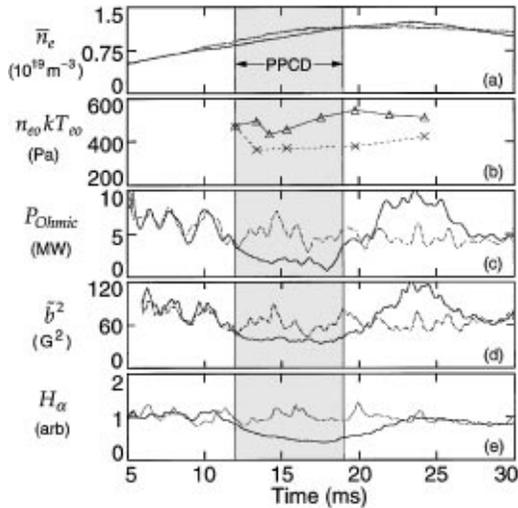
FIG. 3. Shot-averaged wave forms of (a) the central chord line density, (b) central electron pressure from Thomson scattering, (c) Ohmic input power, (d) mean-squared fluctuation amplitude, and (e)  $H_\alpha$  radiation. The unbroken lines are for PPCD plasmas, and the broken lines are for conventional RFP plasmas.
