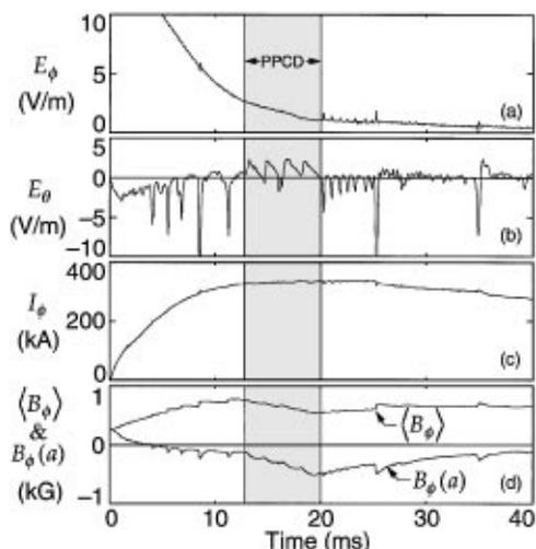
FIG. 1. Wave forms of the (a) surface toroidal electric field, (b) surface poloidal electric field, (c) toroidal plasma current, and (d) average and surface toroidal magnetic field.
