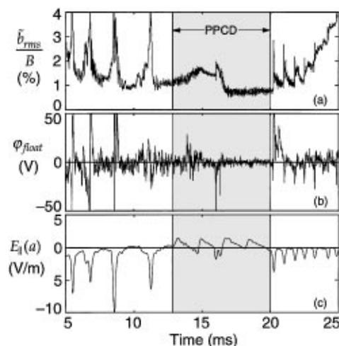
FIG. 2. The (a) spatial root-mean-square magnetic fluctuation, (b) edge floating Langmuir probe voltage, and (c) parallel electric field measured at the plasma surface during improved PPCD.
