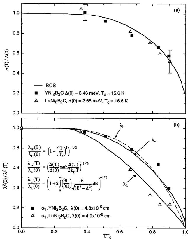
FIG. 3. Temperature dependence of the superconducting energy gap  $\Delta$  (a) and of the penetration depth  $\lambda$  (b) for both compounds, compared with the BCS prediction ( $\lambda_\infty$ ), the London model ( $\lambda_L$ ), and the two fluid approach ( $\lambda_{tf}$ ).
