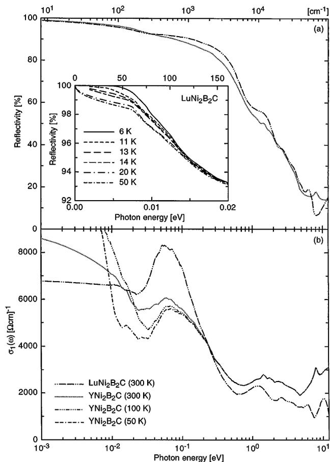
FIG. 1. (a) Reflectivity  $R(\omega)$  and (b) real part  $\sigma_1(\omega)$  of the optical conductivity at 300 K for the Lu and Y compounds over the whole measured frequency spectral range (logarithmic energy scale). For the Y compound the  $\sigma_1(\omega)$  spectra at 50 and 100 K are also displayed. The inset shows the temperature dependence of  $R(\omega)$  in FIR for the Lu compound.
