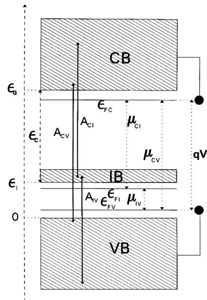
FIG. 1. Band diagram of a solar cell with an intermediate band.
