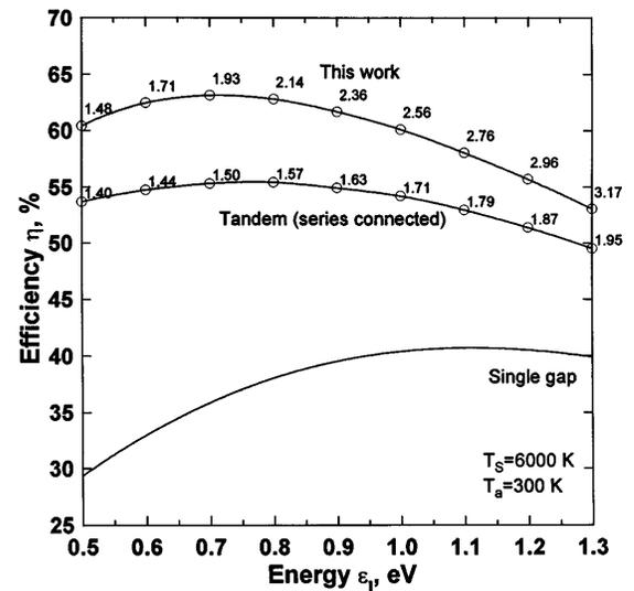
FIG. 2. Efficiency limit for a solar cell with an intermediate band and for a two-terminal ideal tandem cell, in both cases vs the lowest band gap  $\epsilon_I$ , and for a cell with a single band gap. The corresponding values of the highest band gap in cells with intermediate band ( $\epsilon_G$ ) and in tandem cells ( $\epsilon_C$ ), for maximum efficiency, are also presented.
