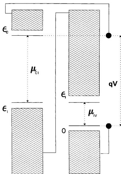
FIG. 3. Band diagram of a two-terminal tandem cell.
