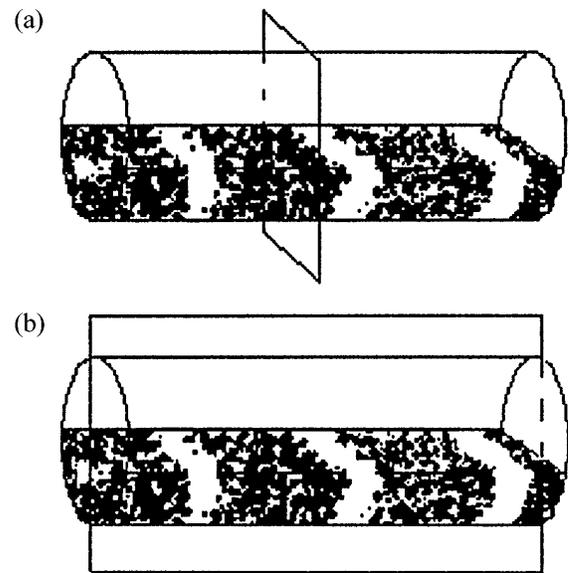
FIG. 1. Sketch of the axial segregation effect in a horizontal cylinder, indicating the orientations of the MRI images used. Both were vertical; one was perpendicular to the axis of the cylinder (a), while the other was parallel to and contained the axis of the cylinder (b). The former was taken at various positions along the length of the tube.
