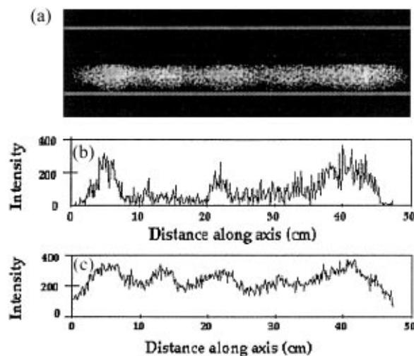
FIG. 3. Data from MRI image parallel to the axis of the cylinder (a) of a mixture of 1 mm pharmaceutical and 3 mm plastic spheres after 9 min of rotation in a 45 cm tube. (b) MRI intensity along the top surface of the system, verifying three axial bands of small spheres as seen from outside the cylinder. (c) Average intensity as a function of position along the axis, from the image shown in (a), indicating five regions of a high concentration of small spheres.
