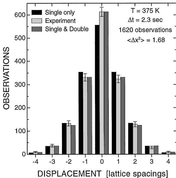
FIG. 2. Distribution of displacements for the self-diffusion of Pt on Pt(110)-(1 × 2) at 375 K. The best fit (dark gray) is obtained with a double to single jump ratio  $h_2/h_1 = 9.5\%$ . The distribution corresponding to diffusion by single jumps only is shown in black.
