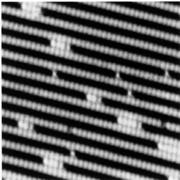
FIG. 1. STM image showing the Pt(110)-( $1 \times 2$ ) surface after a submonolayer amount of Pt has been deposited at 313 K. The presence of single adatoms as well as nucleated islands in the troughs of the missing row reconstruction are evidence for a low thermal mobility ( $97 \times 102 \text{ \AA}^2$ ).
