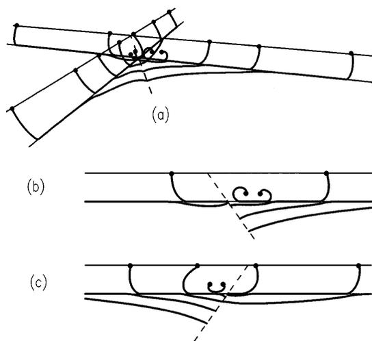
FIG. 3. Typical configuration produced by two Frank-Read sources on intersecting glide planes. The calculation was carried out for a film 5000 Å thick, under a strain of  $4.00 \times 10^{-3}$ . Dots denote the terminations of dislocations on the free surface of the layer or on the pinning sites defining the sources [8]. (a) Perspective view similar to Fig. 1(b). (b) View along the  $[110]$  direction. (c) View along the  $[110]$  direction.
