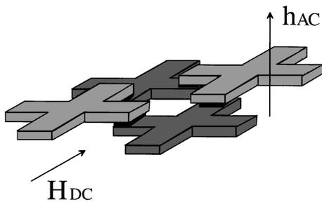
FIG. 2. Sketch of a small section of a sample. The crosses are the niobium islands. The junctions are in the overlap region between these islands.
